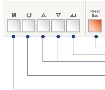
Reset/ESC: Fault reset or ESC from menu
