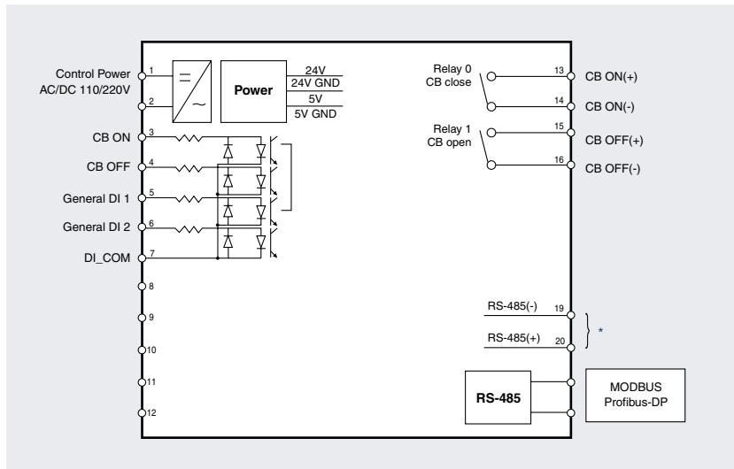
\*In case of using Profibus-DP communication, it needs to communicate with ACB trip relay.
