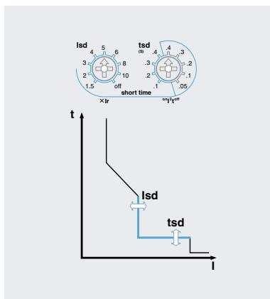
The function for fault current (over current) protection which has definite time characteristic and time delayed in inverse ratio to fault current.
