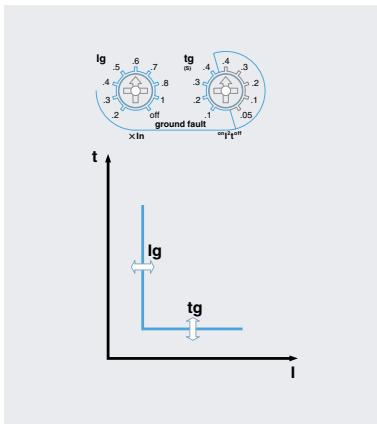
**The function for breaking ground fault current above setting value after time-delay to protect the circuit from ground fault.**
