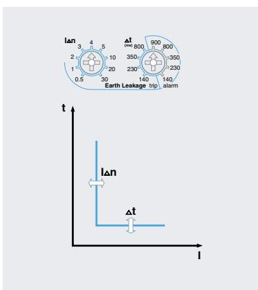
**The function for breaking earth leakage current above setting value after time delay to protect the circuit from earth leakage. (A, P, S type)**
