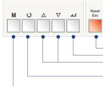
Reset/ESC: Fault reset or ESC from menu
