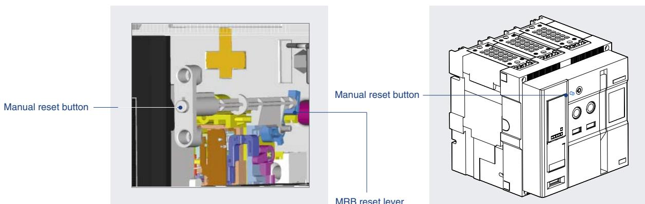
Note) The manual reset button is protruded in the event of trip.
