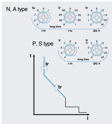
The function for overload protection which has time delayed characteristic in inverse ratio to fault current.
