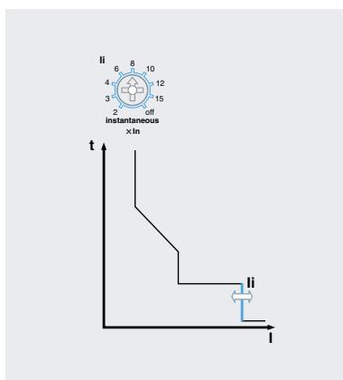
The function for breaking fault current above the setting value within the shortest time to protect the circuit from short-circuit.
